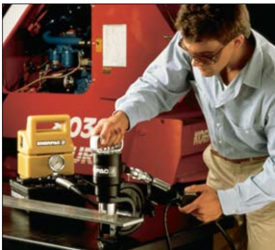
◀ This PUD-1100B is shown with the 35 ton punch and optional gauge.
