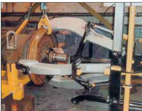
◀ The EPH-1003E quickly and easily removes this drive sheave from its shaft.
