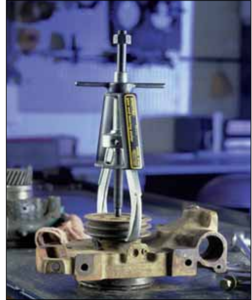
▲ EP-204 2 jaw puller positioned to pull a water pump.
