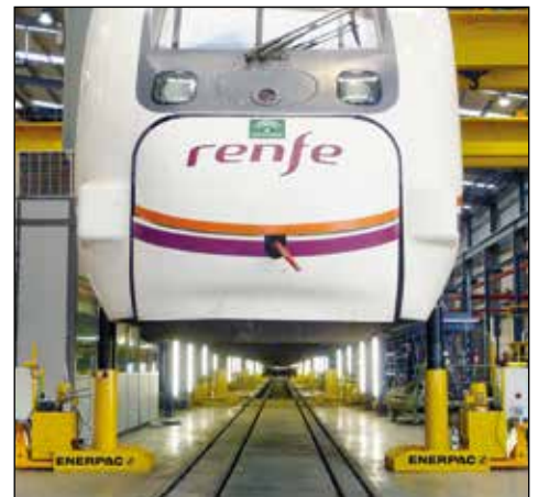
▼ 20-points wireless PLC-controlled train lifting system for rail carriage production and maintenance.
